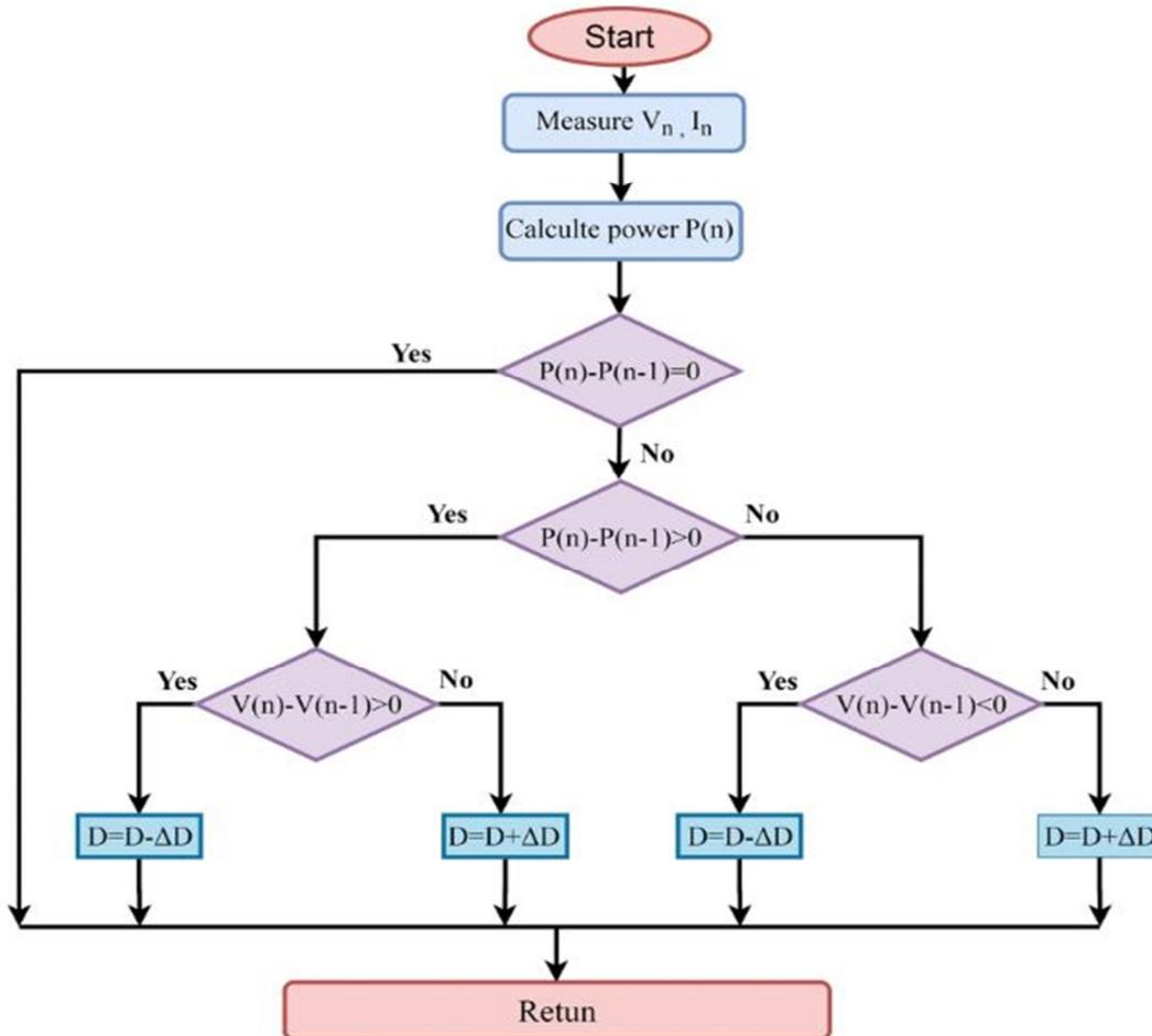
Fig. 3. The Flowchart of the P&O Algorithm [8]
