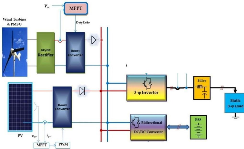
Fig. 1. Block Diagram of Hybrid Solar Wind Power System
