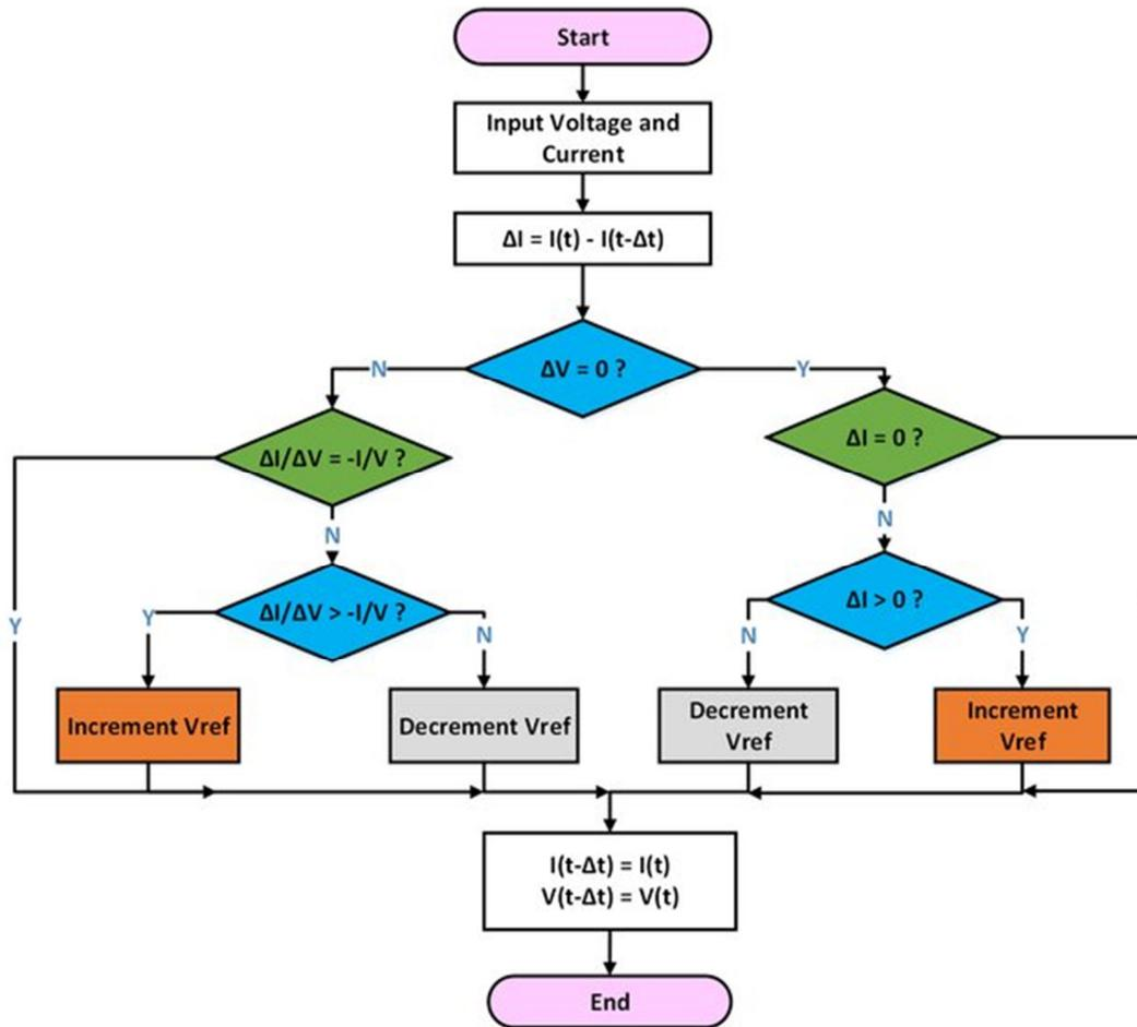
Fig. 4. The Flowchart of the Incremental Conductance Algorithm
