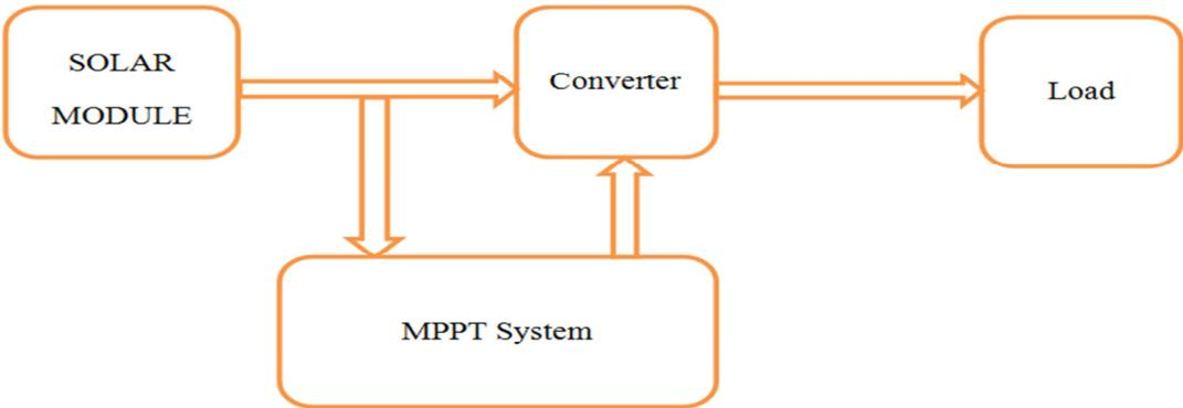
Fig. 2. Block Diagram of MPP Tracking for Solar System
